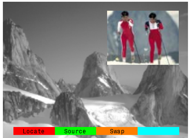
Above, the PIP picture has been moved to an alternative position by pressing the red key.
